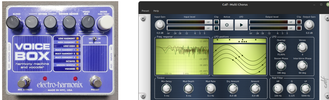
Figure 1.1: A voice processing effect pedal (left) and a digital Chorus plugin (right).
